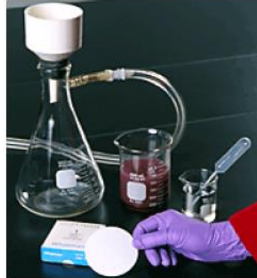
Harvesting (water: filtration)
